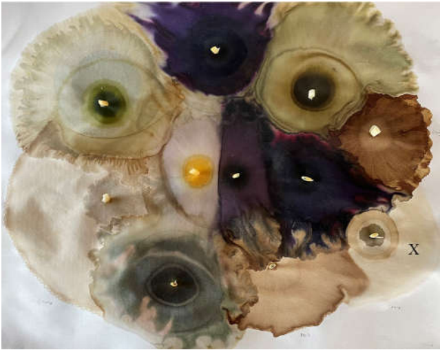
4a. Stiegbildmethode Cartography . Figure with filter wicks, during secondary infiltration with iron sulphate. Capillary Dynamolisis workshop, Cal Franciscano. The colours manifested with iron sulphate are softer but not as fugitive as those filtered through silver nitrate. Photography: Z46.
